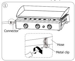
Connect the hose from the griddle to the regulator. Secure the connection with the metal clip on the hose.
