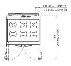
All dimensions in mm; Height is identical on castors
