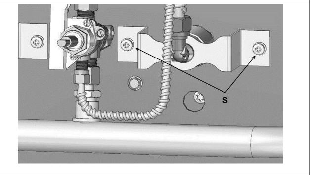
Remove the screws S from the bracket Loosen the the burner feed pipe nut at the valve, this will allow the pipe and bracket to swive
