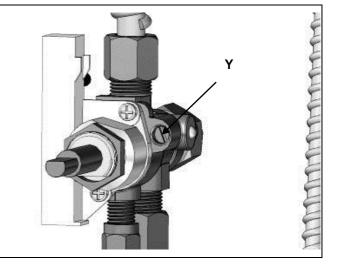
When converting to Propane an external regulator must be fitted to the appliance gas inlet in conjunction with a barrel nipple and or ½" BSP Male-Female 90° elbow NP01 – Barrel nipple CO136 – 90° male/female elbow PG10 - Regulator
