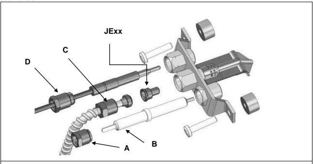
To change the pilot injector very carefully loosen the ignitor retaining nut A and withdraw the ignitor B Loosen and the pilot feed pipe nut C and withdraw the pilot feed pipe from the pilot assembly The pilot injector, JExx, can be removed and replaced with the appropriate injector applicable to gas type Refit the pilot feed pipe and secure nut C Refit the ignitor B
