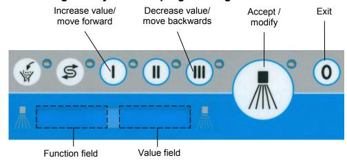
Access codes for various user-levels have been defined. Once the complete code has been entered, the entered code is compared with the internal code table. Depending on the code entered, the corresponding user level will be accessed. 2 access codes are available for each user level; the first is for restricted access, i.e. no modification of parameters is possible (viewing mode), and the second gives access to the entire range of functions (viewing and modification).
