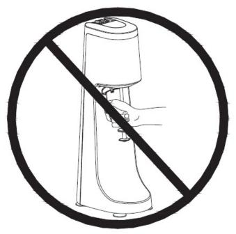
To avoid damage do not lift the mixer by the shaft.
