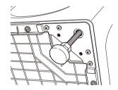
**NOTE:** Keep the leg extension at a minimum to prevent excessive vibration. The more the legs are extended, the greater the machine will vibrate. If the floor is not level or is damaged, you may have to extend the rear leveling legs.
