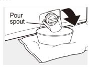
**4.** Turn the pump filter counterclockwise and remove the filter. Open slowly to allow the water to drain.
